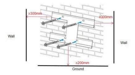
Wall mounting bracket installation
