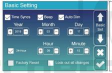
Factory Reset: Reset all parameters of the inverter. Lock out all changes: Enable this menu for setting parameters that require locking and cannot be set up. Before performing a successful factory reset and locking the systems, to keep all changes you need to type in a password to enable the setting. The password for factory settings is 9999 and for lock out is 7777.
