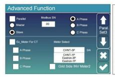
**Ex\_Meter For CT:** when in Three phase system with CHNT Three phase energy meter (DTSU666), click corresponding phase where hybrid inverter is connected. e.g. when the hybrid inverter output connects to A phase, please click A Phase.
