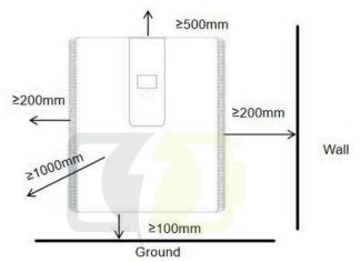
For proper air circulation to dissipate heat, the clearance is about: not less than 200mm on the side, not less than 500mm above, not less than 100mm from the ground, and 100 cm further ahead.
