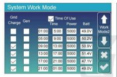
Time of use: it is used to program when to use grid or generator to charge the battery, and when to discharge the battery to power the load. Only tick "Time Of Use" then the follow items (Grid, charge, time, power etc.) will take effect.
