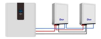
Blue is the network cable, red is the positive electrode, and black is the negative electrode.
