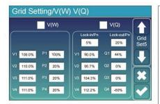
**V(W)**: It is used to adjust the inverter active power according to the set grid voltage.
