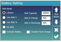
Battery capacity: it tells Deve hybrid inverter to know your battery bank size.
