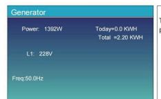
This page tells generator output voltage, frequency, power. And, how much energy is used from generator.
