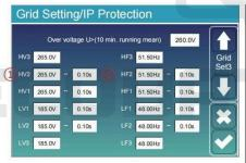
HV1: Level 1 overvoltage protection point;
